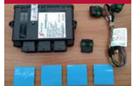
FleetArc Telematics Box Contents w/FA 470 Module
