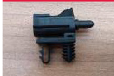
Outside Air Temperature Sensor (OAT - Driver Side)
