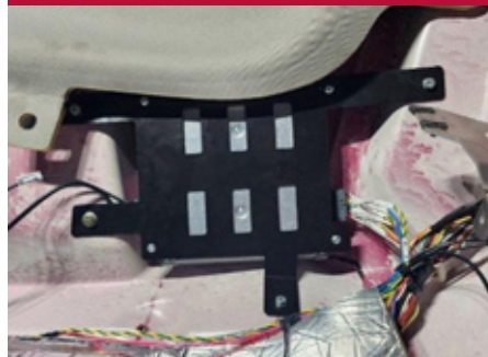
DVR secured to bracket
