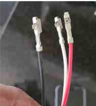
Power, ground, and ignition wires
